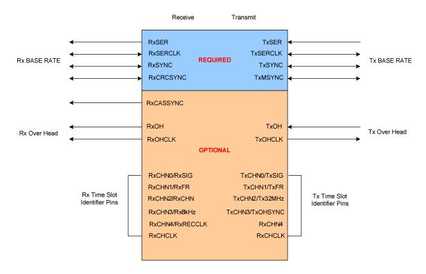
Figure 1. Simplified Block Diagram of One Channel for XRT86VL3x Framer + LIU Combo
